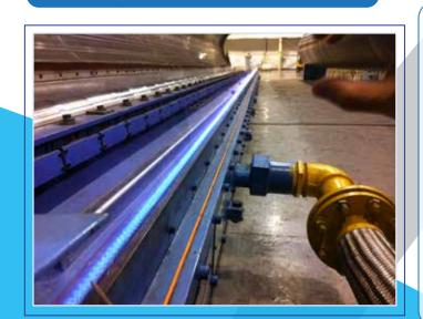
Parex burners supplied for endless felts on PMC (Paper Makers Cloth) machinery.
