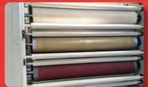
The machine can process with abrasive brushes and emery rollers.
