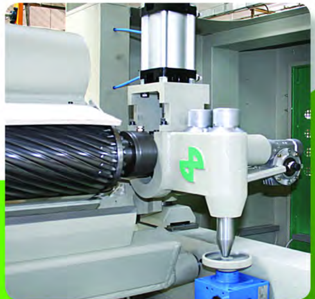
The shearing unit is available with a wide range of shearing blades according to the type of fabric to process.
