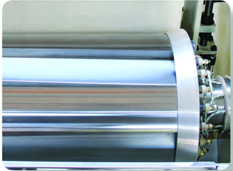
The Polishing roller is made in hard chrome plated steel, with 4 helical grooves. The felt sets the contact between the fabric and the Polishing roller.
